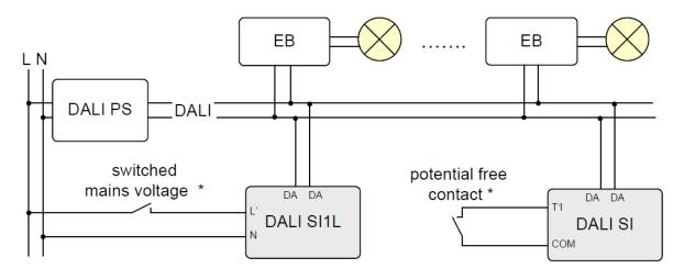
\* typical devices with switching contact: light barrier, motion sensor, relay, switch
